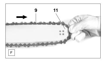
Lead the chain (F/9) around the sprocket nose (F/11) of the guide bar.
